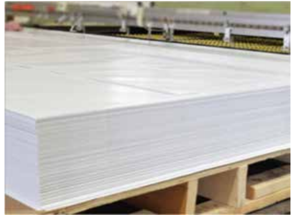
SHEETS OF MEDIA CONDITIONED AND LAYING FLAT DURING PRINTING. (FIG.3)
