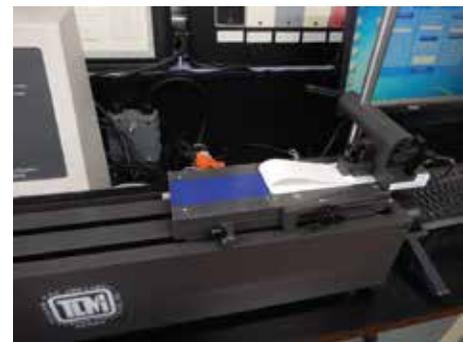
**Low speed 180° Liner Release Test**
