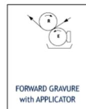
Direct, (forward), or reverse gravure denotes the direction of rotation of the gravure cylinder relative to the movement of the coated substrate. In direct gravure, rotation of the gravure cylinder is in the same direction as the coated substrate. In reverse gravure coating, the gravure cylinder rotates against the direction of substrate movement.
